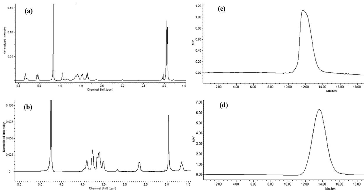
**Fig. 4.** 500 MHz  $^1\text{H-NMR}$  spectrum of *N. meningitidis* polysaccharide recorded in  $\text{D}_2\text{O}$  for serogroup A (a) and serogroup C (b). HPLC profile of *N. meningitidis* polysaccharide eluted with 0.1 M sodium nitrate buffer on TSK 5000-4000 PWXL columns for serogroup A (c) and serogroup C (d), data recorded using RI detector.
