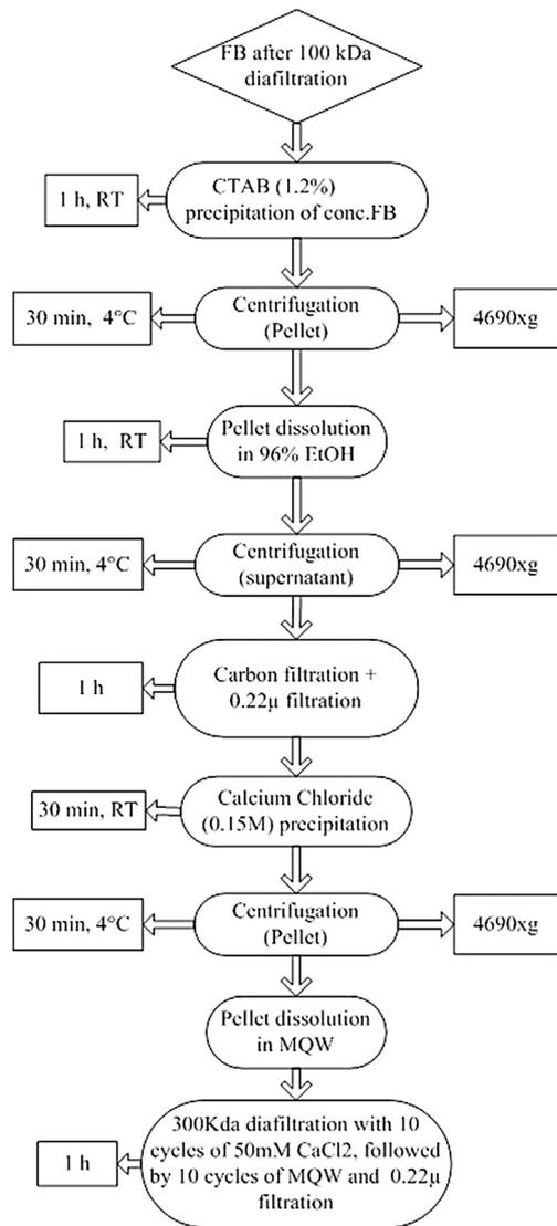
**Fig. 2.** Purification process flow for *N. meningitidis* serogroup A polysaccharide; FB: Fermentation broth; h: Hour; RT: Room temperature; MQW: MilliQ water; Conc.: Concentrated; min: Minutes; EtOH: Ethanol; CaCl<sub>2</sub>: Calcium chloride.
