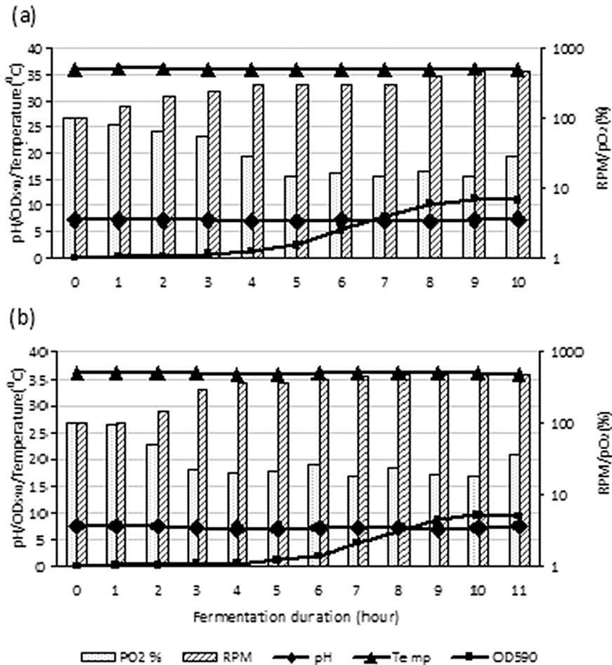
**Fig. 1.** Fermentation parameters and bacterial growth curves for *N. meningitidis* serogroup A (a) and serogroup C (b); OD<sub>590</sub>: Optical density at 590 nm; RPM: Revolutions per minute; pO<sub>2</sub>: Dissolved oxygen; Temp: Temperature.
